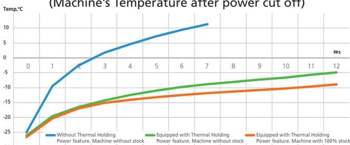
Ice cream temperature would be 2°C to 5°C lower than machine temperature.
